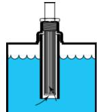
The tank mounted strainer can also be used as an "in-line" strainer with a simple modification. Using standard pipe fittings a "housing" for a strainer can quickly be made and threaded in-line between the
